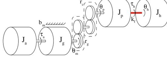
**Fig. 2.** Dynamic model of HANDSON-SEA**Table 1.** Parameters
