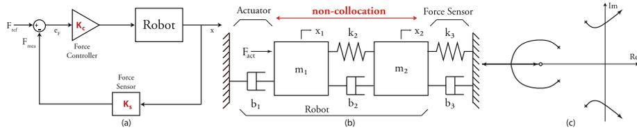
**Fig. 5.** (a) Explicit force controller (b) Linear dynamic model capturing the non-collocation between the sensor and the actuator (c) Representative root-locus plot non-collocated system under explicit force control
